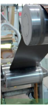
The PVC resin and the additives being provided from the best suppliers to our raw material warehouse and then transferred to the fully automated raw material mixing section without any compromise in the standard formulation and without any manual interference. Then the mixed batch transferred to coloring section, which then passes to the sheet extrusion calendering section.
